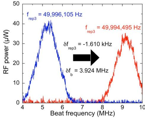
Fig. 12. Spectra of  $f_b$  beat signal when  $f_{\text{rep}3}$  is set at 499 961 05 Hz (blue curve) Hz and 499 944 95 Hz (red curve) (RBW = 10 kHz, sweep time = 189 ms, number of integrated signals = 100).
