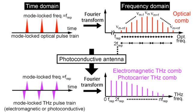
Fig. 1. Optical comb and THz comb.
