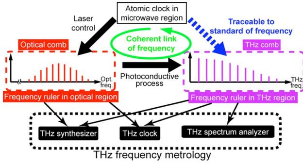
Fig. 2. Coherent link of frequency using frequency comb.
