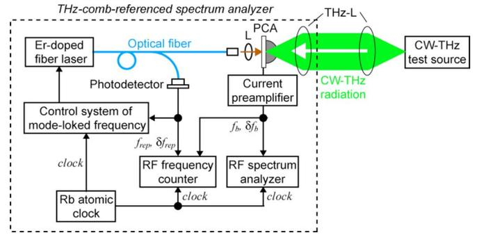
Fig. 4. Experimental setup of THz-comb-referenced spectrum analyzer. L: lens; PCA: bowtie-shaped, low-temperature-grown InGaAs/InAlAs PCA; THz-L: THz lenses.
