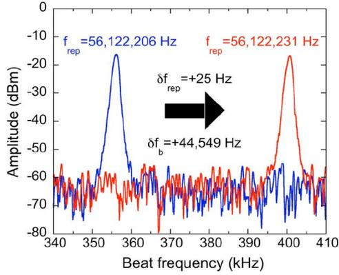
Fig. 6. Spectra of the  $f_b$  beat signal when the laser mode-locked frequency ( $f_{\text{rep}}$ ) is set at 561 222 06 (blue curve) Hz and 561 222 31 Hz (red curve) (RBW = 1 kHz and sweep time = 902 ms).
