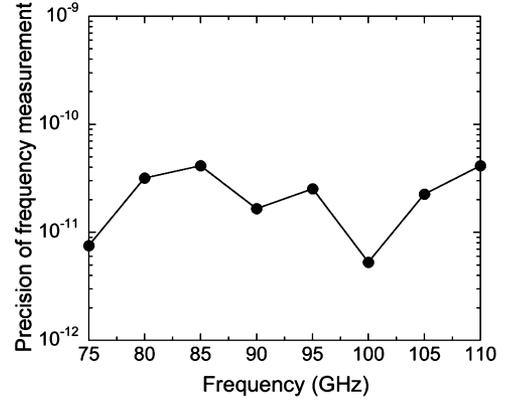
Fig. 7. Precision of frequency measurement in available frequency range of the AFMC source.
