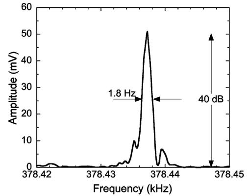
Fig. 5. Spectra of the  $f_b$  beat signal of the AFMC source measured by the RF spectrum analyzer (RBW = 1 Hz and sweep time = 690 ms).
