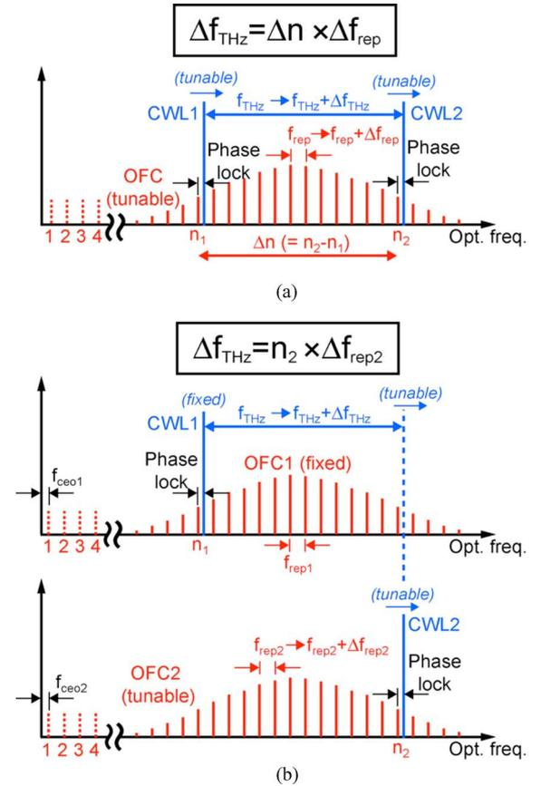
Fig. 10. Continuous tuning of the CW-THz wave based on photomixing of (a) two CW lasers (CWL1 and CWL2) referenced to a single OFC and (b) two CW lasers (CWL1 and CWL2) referenced to two independent optical combs (OFC1 and OFC2).
