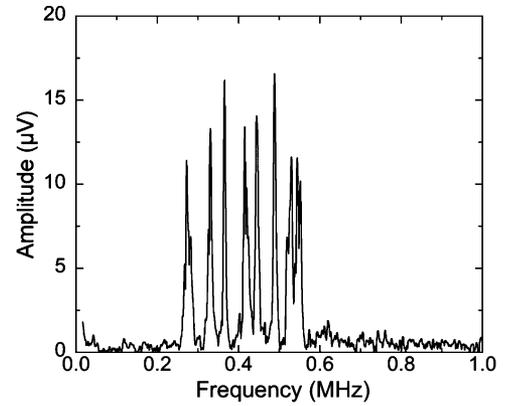
Fig. 8. Spectrum of the  $f_b$  beat signal of the photomixing source (RBW = 1 kHz and sweep time = 13 ms).
