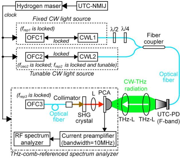
Fig. 11. Experimental setup of continuously tunable, single-frequency CW-THz generator. OFC1, OFC2, and OFC3: OFCs; CWL1 and CWL2: CW near-IR lasers;  $\lambda/2$ : half-wave plate;  $\lambda/4$ : quarter-wave plate; UTC-PD for photomixing; L: lenses; PCA: bowtie-shaped, low-temperature-grown GaAs PCA; THz-L: THz lenses; SHG crystal; UTC-NMIJ.
