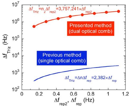
Fig. 14. Relationship between change of  $f_{\text{rep}2}$  or  $f_{\text{rep}}$  ( $\Delta f_{\text{rep}2}$  or  $\Delta f_{\text{rep}}$ ) and that of  $f_{\text{THz}}$  ( $\Delta f_{\text{THz}}$ ) for the presented method, using a dual optical comb, and the previous method, using a single optical comb.
