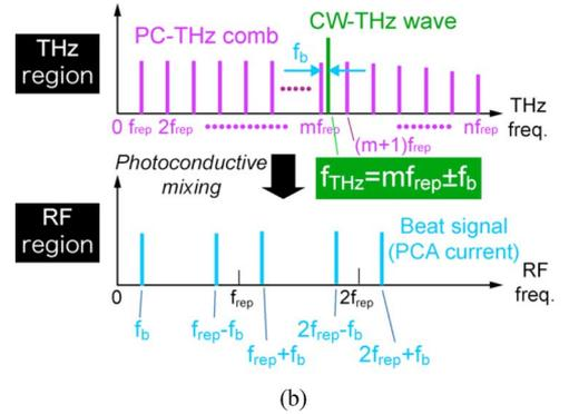
Fig. 3. (a) Principle of THz-comb-referenced spectrum analyzer and (b) corresponding spectral behavior in THz and RF regions.
