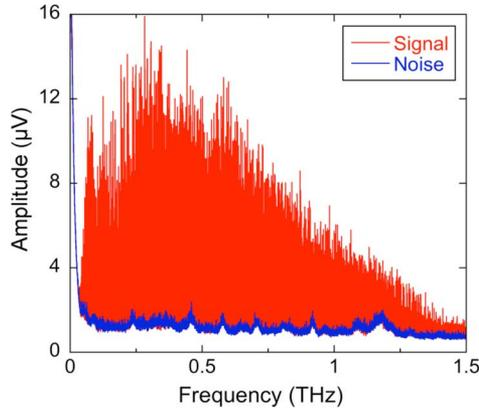
Fig. 9. Spectrum of the EM-THz comb (RBW = 1 kHz and sweep time = 1000 s).
