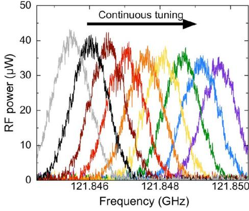
Fig. 13. Continuous tuning of the CW-THz wave around 121.85 GHz by scanning  $f_{\text{rep}2}$  at 0.14-Hz intervals (RBW = 10 kHz, sweep time = 189 ms, number of integrated signals = 100).
