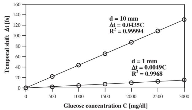
Fig. 3. Relationship between the glucose concentration and the temporal shift in 10-mm cell and 1-mm cell. Measurements were repeated 10 times at each concentration. Solid lines are correlation curve obtained by a linear fitting.
