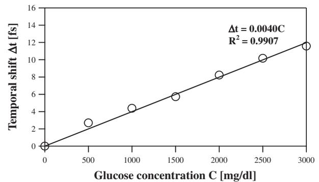
Fig. 5. Relationship between the glucose concentration and the temporal shift in a mixture of a 1.0% intralipid solution and glucose. Thickness of a sample cell is 1 mm. Measurements were repeated 10 times at each concentration. Solid line is a correlation curve obtained by a linear fitting.
