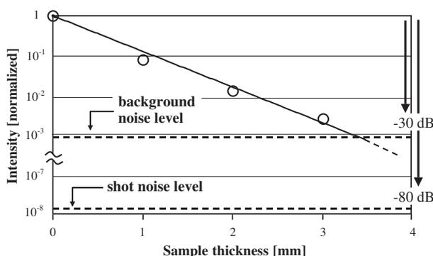
Fig. 4. Maximum intensity of envelope signal detected at each scattering sample thickness. A 1.0% intralipid solution was used as a scattering sample.
