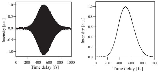
Fig. 3. Interference signal in FTPI: (a) interference fringe signal and (b) extracted envelope signal.
