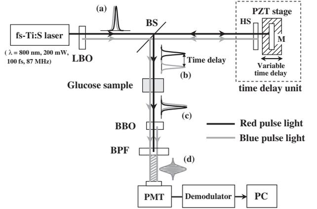
Fig. 2. Experimental setup of FTPI. LBO: frequency-doubling  $\text{LiB}_3\text{O}_5$  crystal, BS: beam splitter, HS: harmonic separator, M: mirror, PZT stage: piezoelectric stage, BBO: frequency-doubling  $\beta\text{-BaB}_2\text{O}_4$  crystal, BPF: blue-pass filter, PMT: photomultiplier, PC: personal computer.
