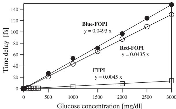
Fig. 4. Relationship between glucose concentration and time delay with respect to red-FOPI, blue-FOPI, and FTPI. Sample thickness is 10 mm. Solid lines are correlation curves obtained by a linear fitting.
