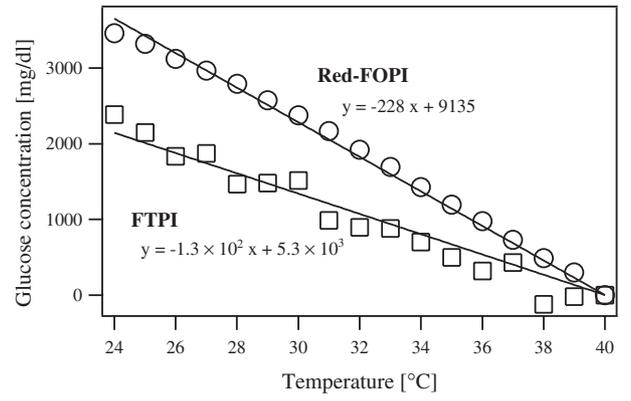
Fig. 5. Dependence of glucose concentration on sample temperature for red-FOPI and FTPI. Sample is pure water with 10 mm thickness. Time delay at  $40^\circ\text{C}$  is defined as origin of time delay fluctuation.
