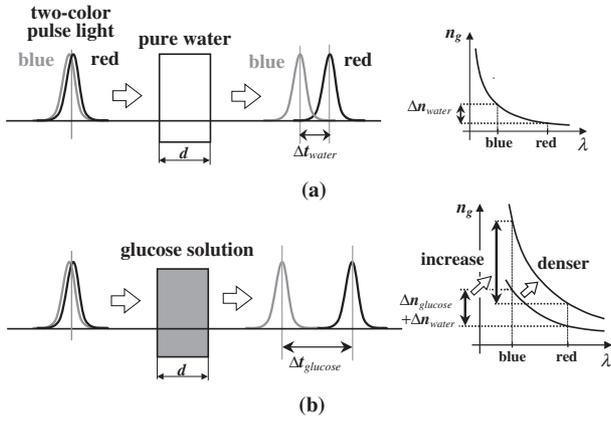
Fig. 1. Glucose concentration measurement based on FTPI: (a) pure water sample and (b) glucose solution sample. When temporally and spatially overlapped two-color (red and blue) pulse is incident to a glucose solution sample, the time delay between the two-color pulse varies depending on the glucose concentration.
