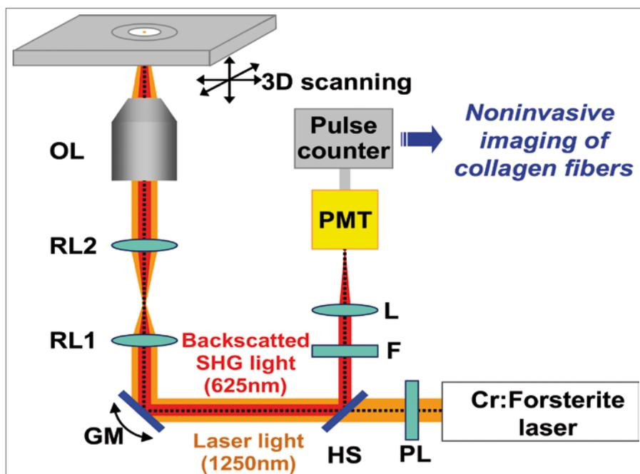
Fig. 3 Experimental setup. PL = polarizer; HS = harmonic separator; F = infrared-cut filter; L = lens, PMT = photomultiplier tube, GM = galvanometer, RL1 and RL2 = relay lens, OL = oil immersion lens
