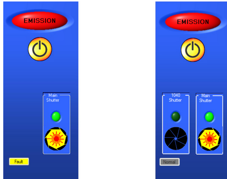
Figure 6-2 Left panel: standard system showing a fault (left), IR option system (right)
