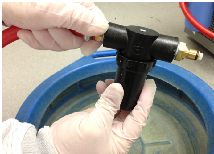
Figure 7-2 Unscrew filter assembly bottom
