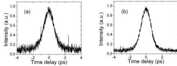
Fig. 5. The autocorrelation trace of (a) 1532.2 nm pulse and (b) 1557.3 nm pulse.
