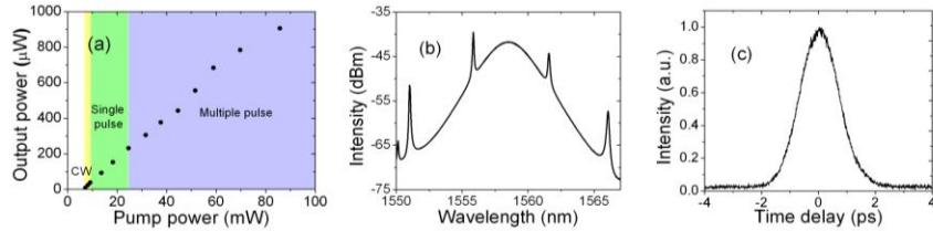
Fig. 2. (a) Output power and operating status of the laser vs. the pump power, when the attenuator is set at 0 dB. (b) Optical spectrum and (c) autocorrelation trace of the laser output centered at  $1558.5 \text{ nm}$  when the pump power is  $16.4 \text{ mW}$ .
