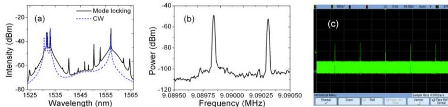
Fig. 4. (a) Output optical spectrum at the dual-wavelength CW and dual-wavelength mode-locked state, when the pump power is 32.8 mW; (b) the corresponding RF spectrum; (c) the corresponding oscilloscope trace.
