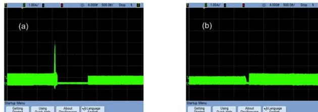
Fig. 6. The oscilloscope trace when mode locking wavelength changes from (a) 1557 nm to 1532 nm and (b) 1532 nm to 1557 nm.
