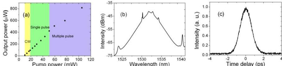
Fig. 3. (a) Output power and operating status of the laser vs. the pump power, when the attenuator is set at 3 dB. (b) Optical spectrum and (c) autocorrelation trace of the laser output centered at  $1532.2 \text{ nm}$  when the pump power is  $19.8 \text{ mW}$ .
