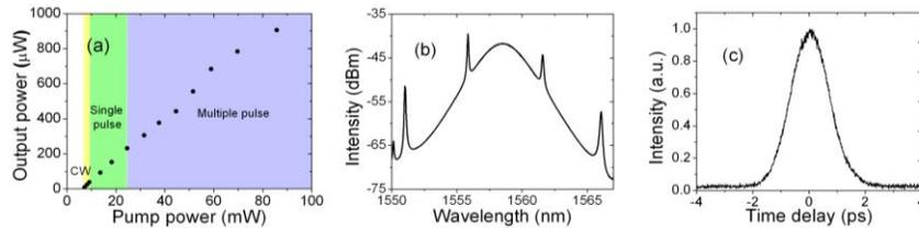
Fig. 2. (a) Output power and operating status of the laser vs. the pump power, when the attenuator is set at 0 dB. (b) Optical spectrum and (c) autocorrelation trace of the laser output centered at 1558.5 nm when the pump power is 16.4 mW.
