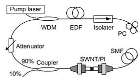
Fig. 1. Schematic of the experimental setup.
