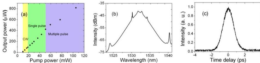
Fig. 3. (a) Output power and operating status of the laser vs. the pump power, when the attenuator is set at 3 dB. (b) Optical spectrum and (c) autocorrelation trace of the laser output centered at 1532.2 nm when the pump power is 19.8 mW.
