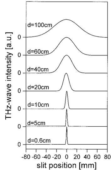
Fig. 3. Intensity cross section of the THz wave in the horizontal direction at distance  $d$  from a single Si-prism coupler. The measured diffraction angle of the THz wave in the far field was 1.4 deg.
