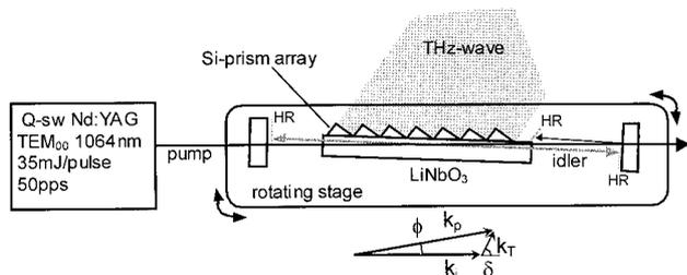
Fig. 1. TPO with a Si-prism array. The Si-prism array was introduced to increase the output and to reduce the diffraction angle of the THz wave by increasing the coupling area. An array of seven right-angle Si-prism couplers was placed on the  $y$  surface of the  $\text{LiNbO}_3$ . The total base length was  $8 \text{ mm} \times 7 = 56 \text{ mm}$ .
