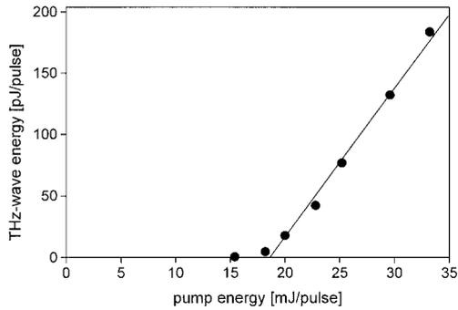
Fig. 2. Typical input-output characteristics of a TPO with a Si-prism array. The THz-wave output increased to greater than six times that of a single-prism coupler because of its wide base.
