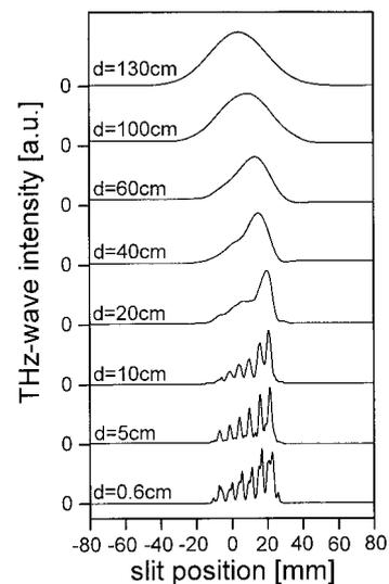
Fig. 4. Intensity cross section of the THz wave in the horizontal direction at distance  $d$  from the Si-prism array. A comparison of the FWHM at  $d = 100$  cm proved that the diameter of the THz wave was 40% smaller than that of a single-prism coupler.
