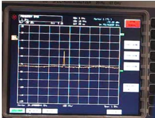
Fig. 6. Metal-metal QCL. (Media 1) Video sample of the SA screen. The RF-power is of  $-2\text{dBm}$ .  $f_{\text{RF}}$  is swept at constant speed from the low frequency side (from left to right on the screen). The frequency scale is of  $100\text{MHz/div}$ . The intensity scale is of  $10\text{dB/div}$ . The oscillations of the intensity of the RF signal are the consequence of an interference effect due to the non-ideal directivity of the coupler shown in Fig. 2 (see text).
