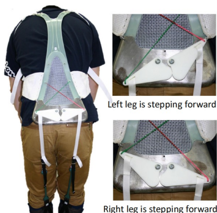
Fig.1 Photo of back assistive device with easy-walk mechanism
