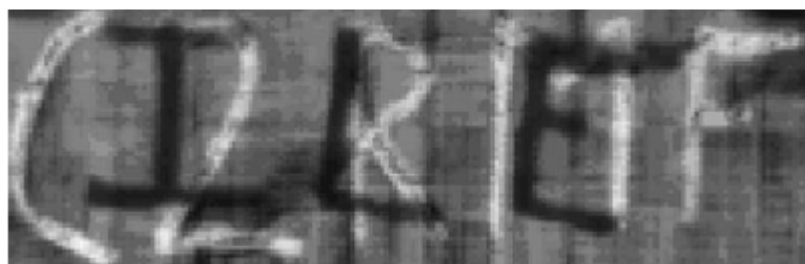
Fig. 8 THz image of second layer of papyrus with a distance of 5 mm, in white the ink and in dark the shadow of the top layer
