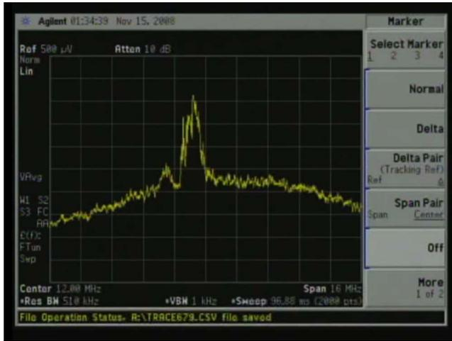
FIG. 4. Real-time monitoring of the phase-locked cw-terahertz radiation when locking its output frequency at 121.847 772 GHz (full span=4 MHz, sweep time=97 ms, and RBW=510 kHz) (enhanced online). [URL: <http://dx.doi.org/10.1063/1.3305324.1>]
