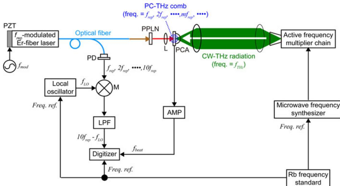
**Fig. 3** Experimental setup for absolute frequency measurement with  $f_{\text{rep}}$ -modulated PC-THz comb. *PPLN* periodically-poled-lithium-niobate crystal, *L* objective lens, *PCA* photoconductive antenna, *PC-THz-comb* photocarrier THz frequency comb, *M* mixer, *LPF* low-pass filter, *AMP* current preamplifier
