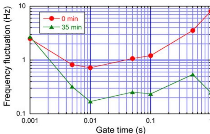
**Fig. 7** Frequency fluctuation of unstabilized  $f_{\text{rep}}$  at different gate time immediately after switching on the femtosecond laser (0 min) and 35 min later
