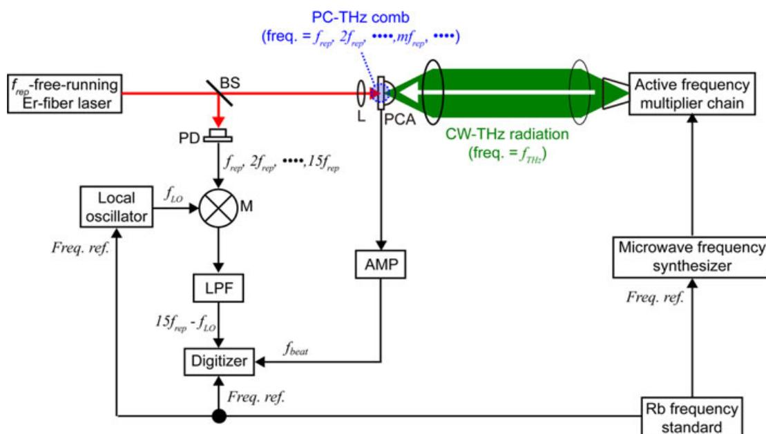
**Fig. 4** Experimental setup for absolute frequency measurement with  $f_{\text{rep}}$ -free-running PC-THz comb. BS beam splitter, L objective lens, PCA photoconductive antenna, PC-THz-comb photocarrier THz frequency comb, M mixer, LPF low-pass filter, AMP current preamplifier
