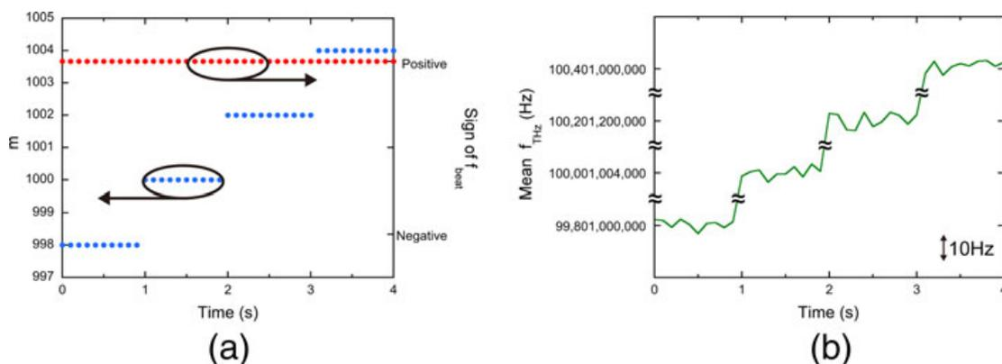
**Fig. 6** Temporal changes of **a** the value of  $m$  and the sign of  $f_{\text{beat}}$  and **b**  $f_{\text{THz}}$  when  $f_{\text{THz}}$  was made to stepwise jump at intervals of +200 MHz four times from 99,801,000,000 Hz to 100,401,000,000 Hz during 4 s. The measurement rate was 10 Hz
