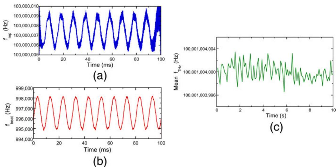
**Fig. 5** Temporal changes of instantaneous values of **a**  $f_{\text{rep}}$  and **b**  $f_{\text{beat}}$  for measurement time of 100 ms. **c** Temporal changes of  $f_{\text{THz}}$  determined at a measurement rate of 10 Hz for a measurement time of 10 s
