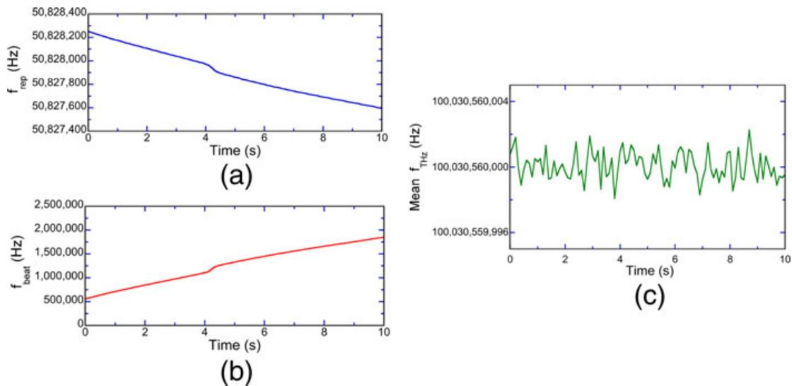
**Fig. 8** **a** Temporal changes of instantaneous values of **a**  $f_{rep}$  and **b**  $f_{beat}$  for a measurement time of 10 s. **c** Temporal changes of  $f_{THz}$  determined at a measurement rate of 10 Hz for a measurement time of 10 s
