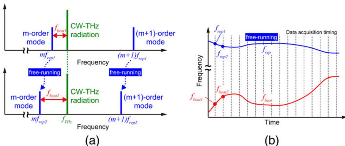
**Fig. 2** Principle of real-time measurement with  $f_{\text{rep}}$ -free-running PC-THz comb. **a** Spectral behavior of  $f_{\text{rep}}$ -free-running PC-THz comb and a measured CW-THz radiation and **b** the corresponding description of  $f_{\text{rep}}$  and  $f_{\text{beat}}$  in the time domain
