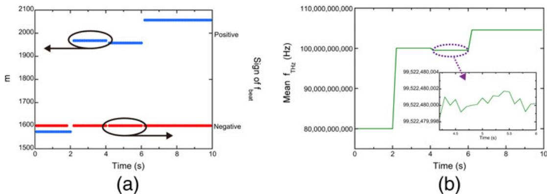
**Fig. 9** Temporal changes of **a** the value of  $m$  and the sign of  $f_{beat}$  and **b**  $f_{THz}$  when  $f_{THz}$  was made to stepwise jump at intervals of +20 GHz, -500 MHz, and +5 GHz from 80,004,900,000 Hz during 10 s. The measurement rate was 10 Hz
