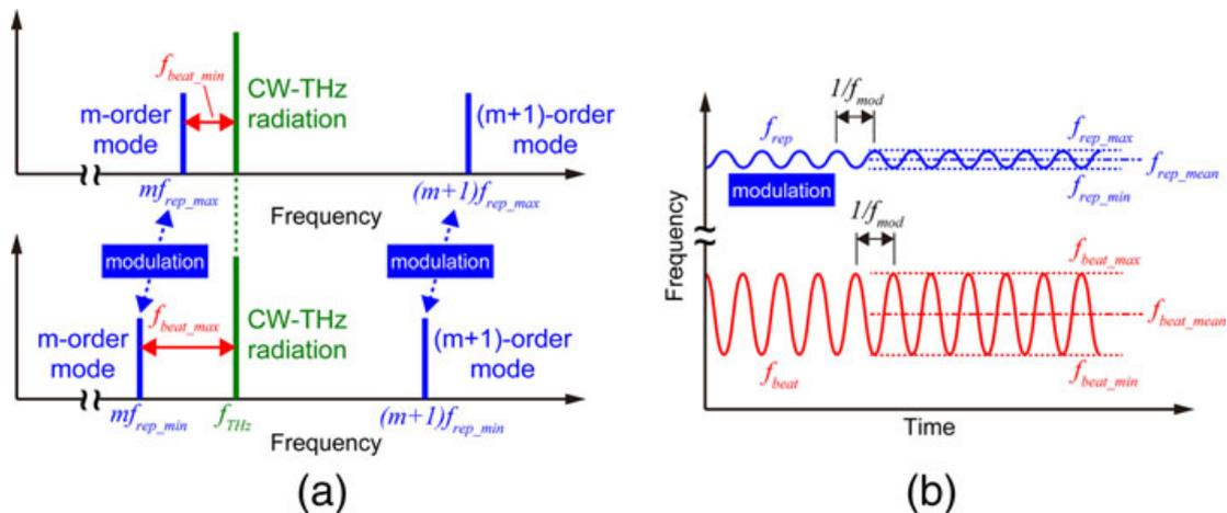
**Fig. 1** Principle of real-time measurement with  $f_{\text{rep}}$ -modulated PC-THz comb. **a** Spectral behavior of  $f_{\text{rep}}$ -modulated PC-THz comb and measured CW-THz radiation and **b** the corresponding description of  $f_{\text{rep}}$  and  $f_{\text{beat}}$  in the time domain
