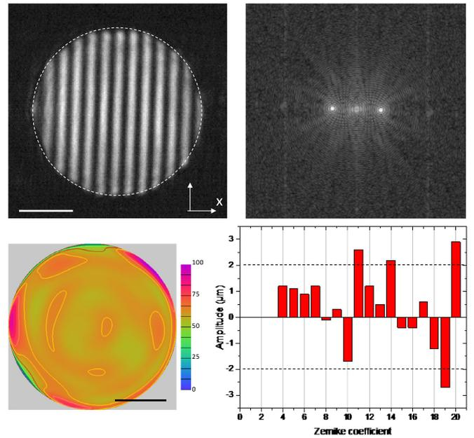
Fig. 2. Optical aberrations delivered by the interferometer. (a) Interferogram. White circle: image selection for FFT analysis. (b) Fourier domain image. (c) Reconstructed wavefront. (d) Amplitude of the Zernike coefficients. Dotted black lines: limits of the measurement.
