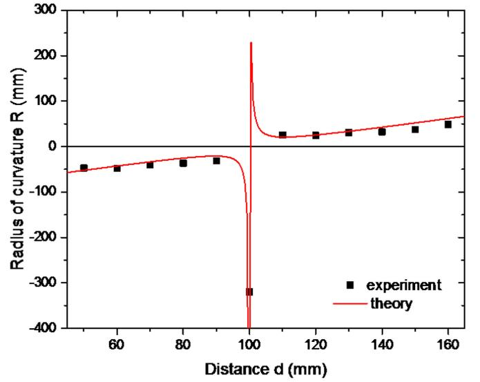
Fig. 6. Evolution of the amplitude of the radius of curvature  $R$  as a function of the distance  $d$  between the lens  $L$  and the pinhole.
