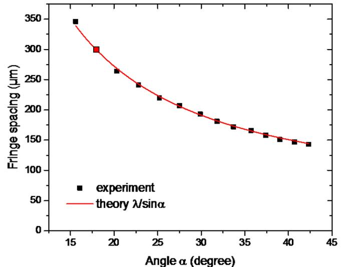
Fig. 3. Evolution of the fringe spacing as a function of the angle  $\alpha$  between the two interfering waves. In the rest of our study, the angle  $\alpha$  was fixed to  $18^\circ$ , indicated by the red square experimental point.
