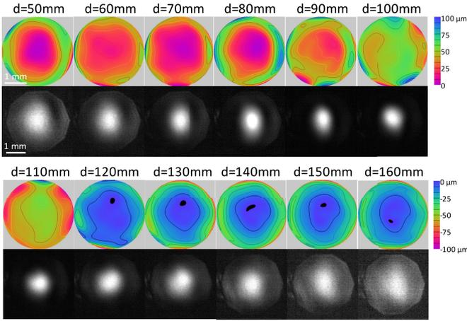
Fig. 5. THz wavefront (color) and THz beam (grey) as a function of the distance  $d$  between the lens  $L$  and the pinhole. The measurements are performed by the THz camera that images the pinhole plane. The distance  $d = 100$  mm corresponds to the theoretical position of the beam waist.
